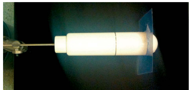
Fig. 2. Measurement setup with dosimetric film fixed perpendicular to the applicator, ready for submersion in the water phantom
