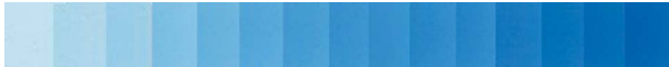
Fig. 4. Digitized sheets of the films used to obtain calibration data. Deposited doses from left to right are: 0.0 Gy, 0.25 Gy, and 0.5-5.0 Gy with 0.5 Gy intervals, and 5-8 Gy with 1.0 Gy intervals
