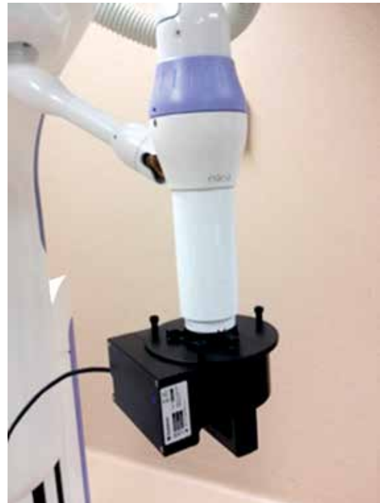
Fig. 2. Setup of the diode QA tool
