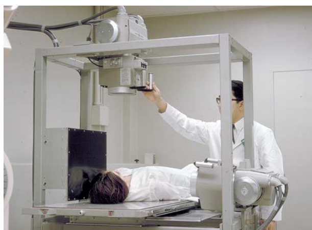
Fig. 5. The stereographic reference frame developed by the Memorial Physics Department to maintain a fixed geometry for stereoshift or orthogonal radiographs. This image was provided courtesy of Stephen Balter
