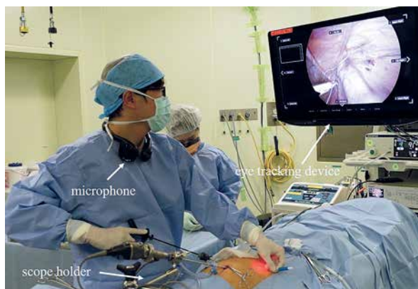
Photo 2. View of the setup. The eye tracking device on the monitor recognizes the surgeon's point of gaze on the image. The surgeon gives voice commands that are received by a microphone, and the image is enlarged and moved around the gazing point accordingly. The endoscope is fixed in a holder, and no scope manipulation is performed by the assistant
